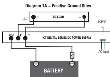
When using the LVD in a positive ground system (Diagram 1A), do not ground the positive terminal of the battery. System must only have a single ground connection, normally located at the power distribution or load point. An additional ground connection at the battery will allow current to bypass the LVD contactor, preventing the disconnection of the battery during a low voltage event.
