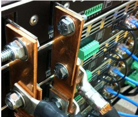
**(Figure: 4 Back Panel Parallel Connections)**
