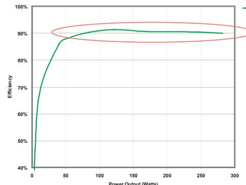
Fig. 4 ICT inverters are designed to run at their highest efficiency across a wide power output range.
